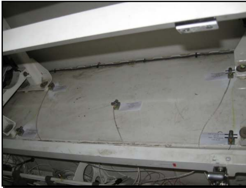
Figure 4. Transducer placement (input to missile rack).
